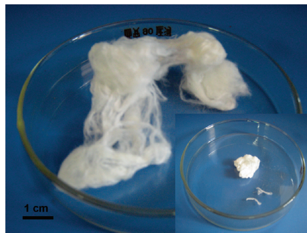
Figure 5. Photographs of the T6 composite fibers and T-400 of the fiber-like TiO 2 nanomaterials (inset).
